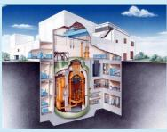
JAEA has been conducting research and development in the HTTR (High-Temperature Engineering Test Reactor) project since 1999, aiming to establish both HTGR technology and technology for nuclear heat applications.
